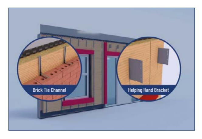
UNipanel<sup>LB</sup> comes complete with the appropriate fixings for your choice of external finish. Every choice can be accommodated, whether you need brick ties for brickwork, helping hand brackets for cladding or a brick slip system, or fixings for a combination of finishes.
