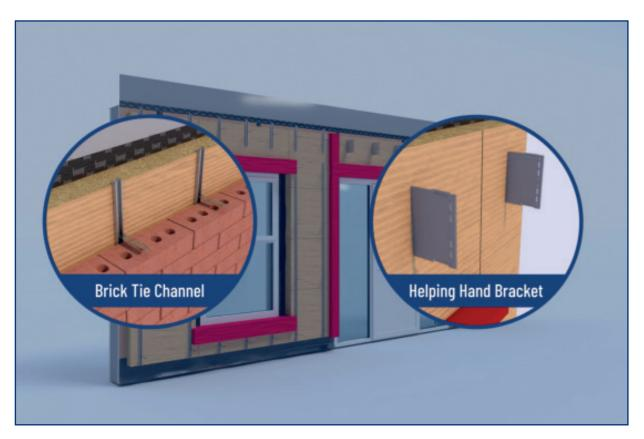
UNIPANEL<sup>LB</sup> CAN BE ADAPTED TO ANY TRADITIONAL SFS DESIGN, WITH FIXINGS APPLIED FOR THE EXTERNAL FINISH OF YOUR CHOICE; BRICK TIES FOR BRICKWORK, HELPING HAND BRACKETS FOR CLADDING OR A BRICK-SLIP SYSTEM, OR BOTH TO SUPPORT A HYBRID AESTETHIC FINISH
