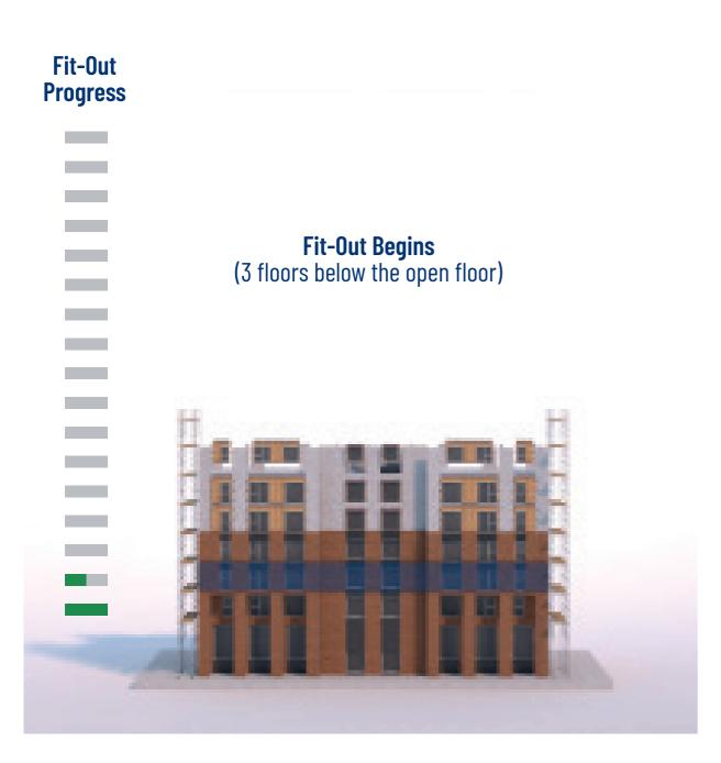
ONCE THE PODIUM HAS BEEN COMPLETED, UNISYSTEM<sup>SFS</sup> IS INSTALLED AS THE CONSTRUCTION OF THE MAIN STRUCTURE PROGRESSES, PROVIDING A WEATHERTIGHT 'DRY BOX' ENVIRONMENT IN A SIGNIFCANTLY SHORTER TIMEFRAME THAN TRADITIONAL BUILD. ONCE THE BUILDING REACHES FOURTH FLOOR PLATE, FIRST FIX CAN BEGIN ON FIRST FLOOR AND FINAL FIX CAN BE COMPLETED RAPIDLY AFTER.
