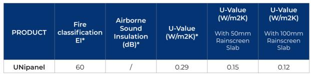
The performance figures provided exclude any finishes. U-values shown are for brickwork construction.
