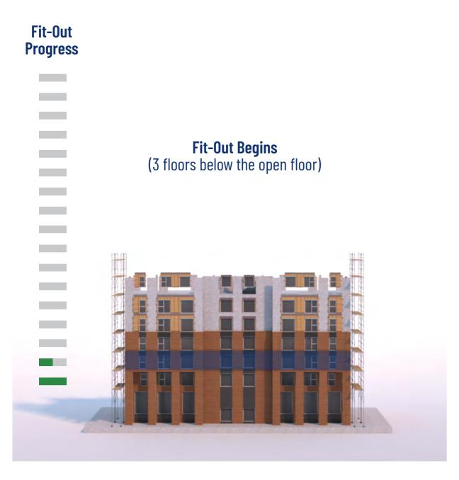
UNIPANEL AND UNIWALL ARE INSTALLED AS THE CONSTRUCTION OF THE MAIN STRUCTURE PROGRESSES, PROVIDING A CLOSED WATERTIGHT ENVIRONMENT IN A FAR SHORTER TIMEFRAME THAN TRADITIONAL BUILD. THIS ENABLES INTERNAL FIT-OUT TO BEGIN THREE FLOORS BELOW THE OPEN FLOOR.
